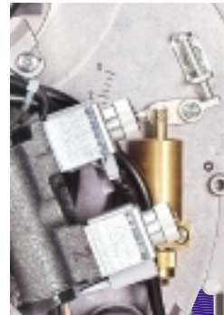
1 st stage air damper adjustment
